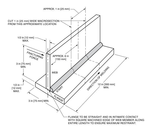
Source: Figure 4 of AWS A5.29/A5.29M:2005 (ERRATA/REPRINT).
