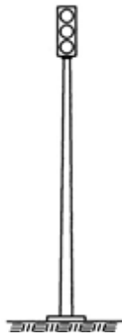
Pole Top-Mounted Traffic Signals
